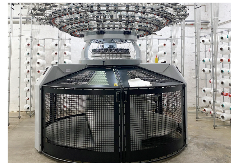
One of Gabriel's circular knitting machines which produces Beyond Loop and other fabrics.
